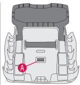
To reposition the crotch strap, first turn the child restraint upside down. Turn the crotch strap harness anchor A sideways and push it through the slot in the bottom of the seat shell **B**.
