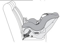
Infants MUST always ride facing the rear of the vehicle. The back of the child restraint supports and protects the baby and absorbs crash forces. Adjust the child restraint to the *Recline* position (p. 18). Place the child restraint in your vehicle rear-facing.
