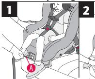
To tighten the harness straps, pull on the long harness adjuster strap (A) on the front of the seat.
