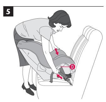
Using your full weight, push the child restraint firmly into the vehicle seat while pulling up on the lower anchor connector assembly strap to tighten.
